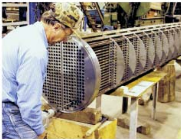
Expanding the tubes into the tubesheet
